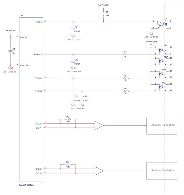
Figure 18 - TA330-E01 Isolation Diagram
