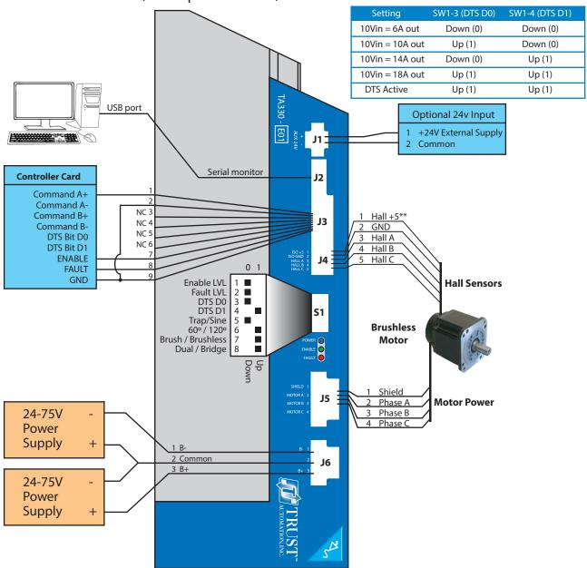
This figure shows the TA330-E01 operating in trapezoidal mode with single ended command input. Active low enable, active low fault, driving a single brushless servo motor, using Hall Effect sensors at 120° timing for trapezoidal commutation. The TA330-E01 is set for a fixed current limit of 14A with a transconductance of 1.4A/V.
