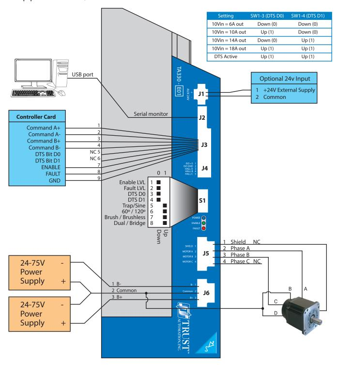
This figure shows the TA330-E01 operating in brushed dual mode with differential command inputs. Active low enable, active low fault, driving a stepper motor sinusoidally. The TA330-E01 is set for a fixed current limit of 6A with a transconductance of 0.6A/V.
