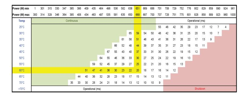
Figure 11 – Temperature Derating, Time to Fault for Dissipation Wattages vs. Heatsink Temperature
