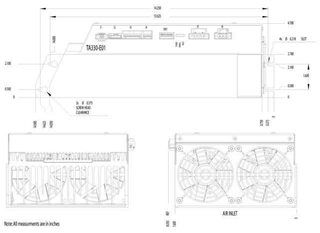
Figure 13 - TA330-E01 Mechanical Dimensions
