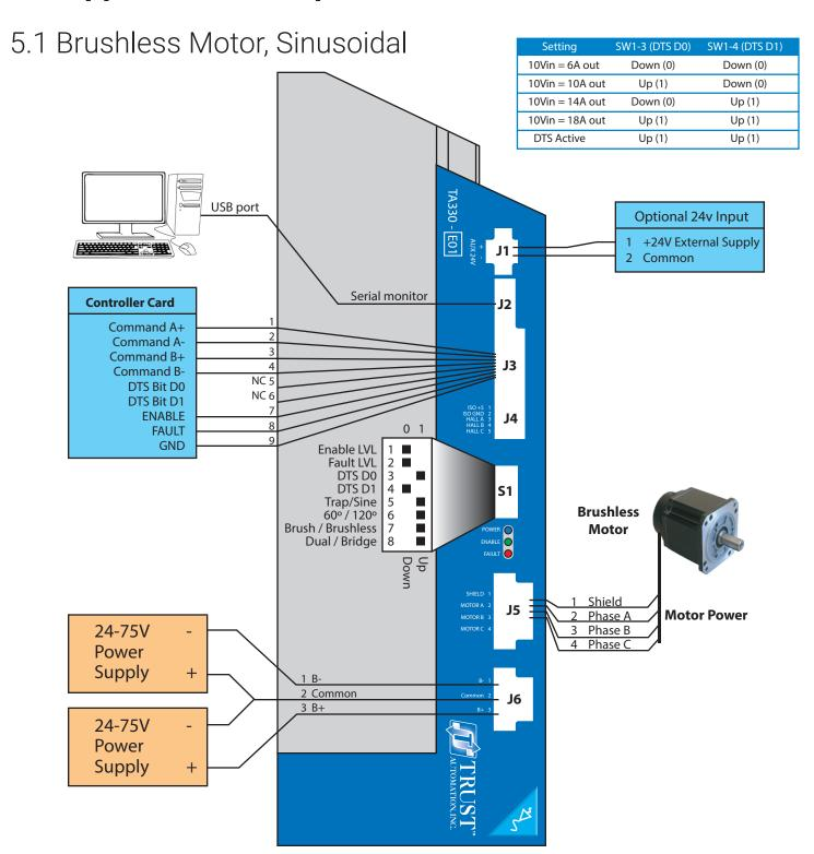
The figure shows the TA330-E01 operating in sinusoidal mode with differential command inputs. Active low enable, active low fault, driving a single brushless servo motor. The TA330-E01 is set for a fixed current limit of 10A with a transconductance of 1.0A/V.
