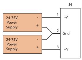
Figure 3 - Drive Power Connection
