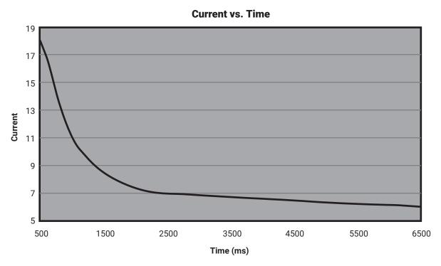
Figure 9 - Output Current vs. Time Graph for Time to Fault at ~30°C
