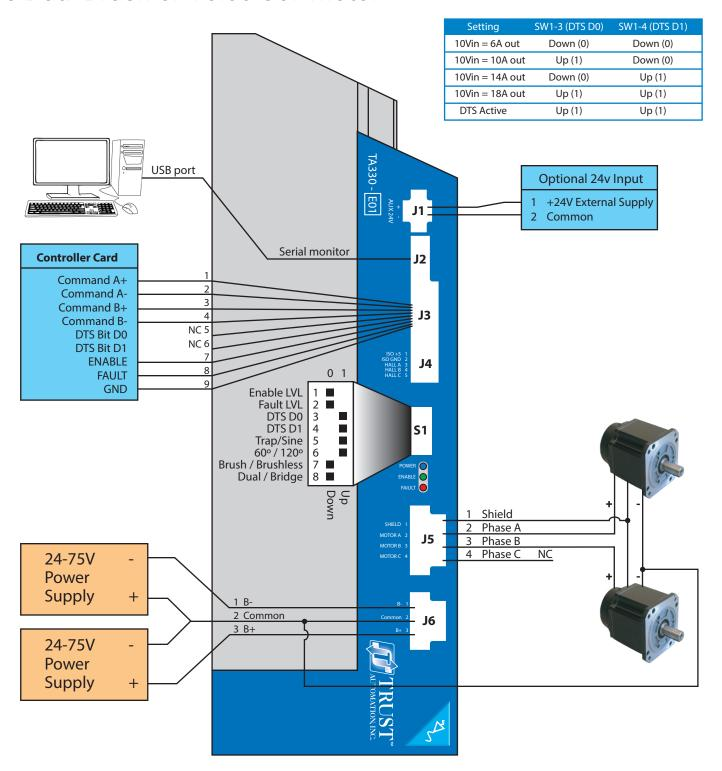
This figure shows the TA330-E01 operating in brushed bridge mode with differential command inputs. Active low enable, active low fault, driving a single brush type servo motor. The TA330-E01 is set for a fixed current limit of 18A with a transconductance of 1.8A/V.
