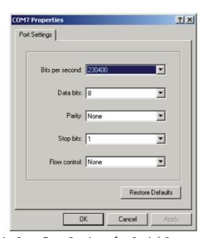
Figure 4 - Com Port Settings for Serial Communication
