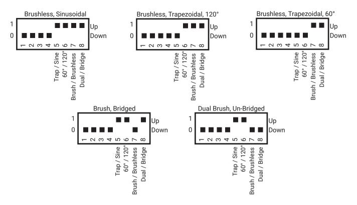
Figure 16 - SW1 Motor Type Settings
