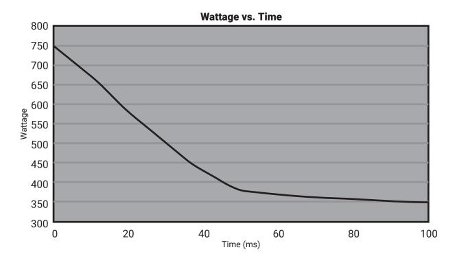
Figure 10 - Dissipation Wattage vs. Time for Time to Fault at ~30°C
