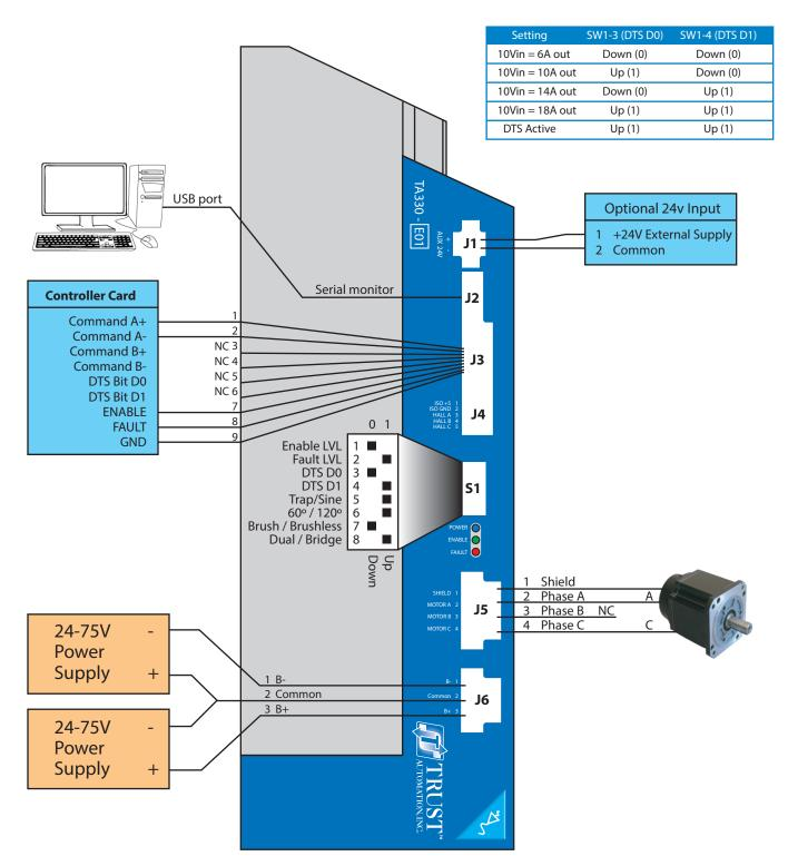
This figure shows the TA330-E01. Active low enable, active high fault, driving a single brushless servo or voice coil motor. The TA330-E01 is set for a fixed current limit of 14A with a transconductance of 1.4A/V
