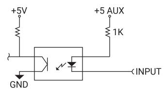
Figure 1 - Enable Circuit
